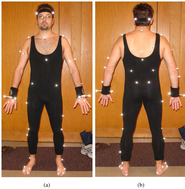
FIGURE 5. The sensors on human body of CMU motion capture database. (a) Sensor Locations from front view. (b) Sensor Locations from back view.
