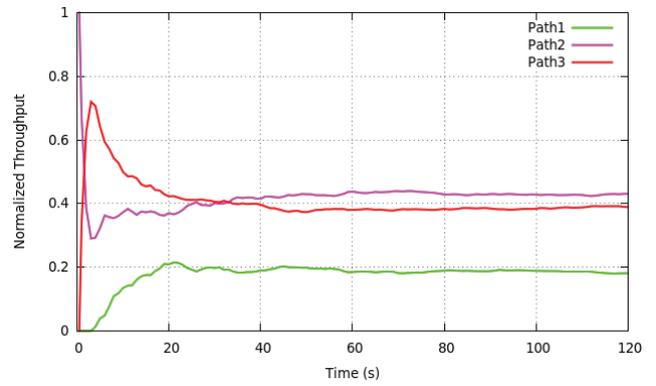
FIGURE 7. Normalized throughput with EEMPTCP.
