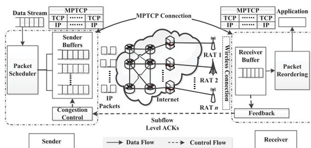
FIGURE 1. System model of multipath communication with MPTCP.
