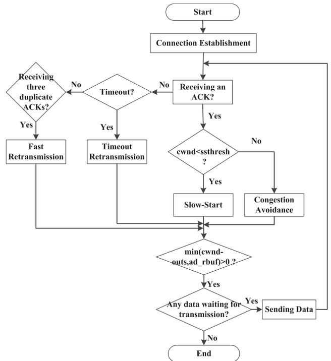
FIGURE 2. Control flowchart of a subflow in the MPTCP connection.
