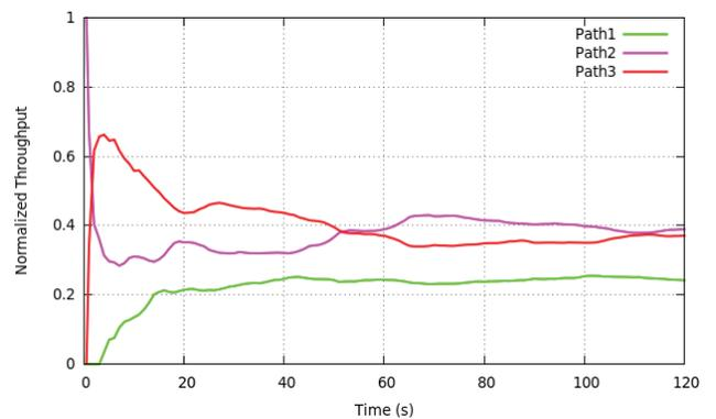
FIGURE 8. Normalized throughput with MPTCP.
