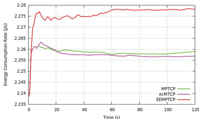
FIGURE 5. Comparison of energy consumption rate.
