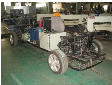
FIGURE 6. The prototype vehicle with active suspension.
