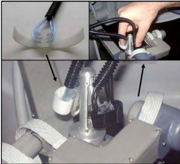
FIGURE 4. Illustration of pneumatic actuators mounted on the da Vinci robotic grasping tool introduced in [29], [70], and [72].
