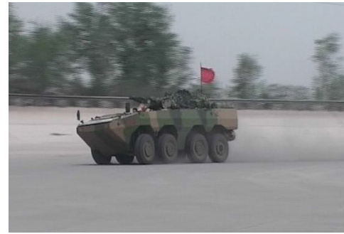
FIGURE 9. Full-sized four-axle HEGV driven by IWMS.
