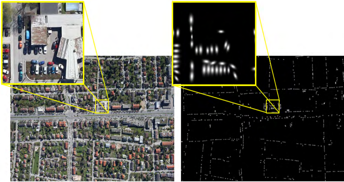
FIGURE 2. Training procedure tries to find a mapping function that maps the input image I(x) to the density map D(x) . (left) Represents the input image I(x) whereas (right) is the density map. Each vehicle is represented by 2-D Gaussian function.
