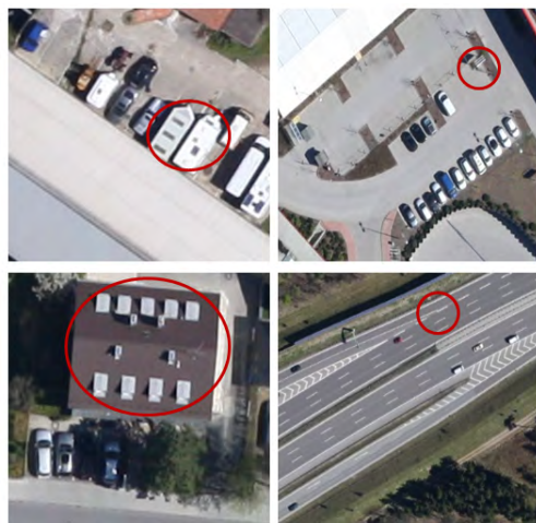
FIGURE 1. Examples of some of vehicle detection challenges (small vehicle sizes, different types and orientations, other similar objects such as air conditioning units on building, trash bins, and road marks) are shown by red ellipses.
