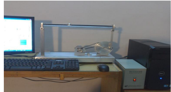
FIGURE 9. Experimental Setup of the Ball and Beam equipped via Googoltech GBB1004.
