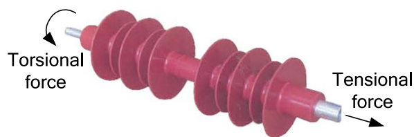
FIGURE 1. Force analysis diagram of the insulator.
