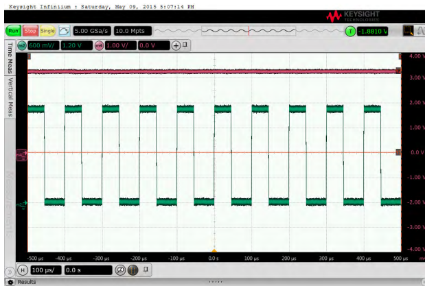
FIGURE 13. Wake-up receiver's ASK demodulation output and wake-up output.
