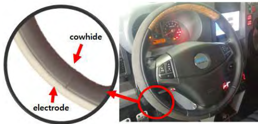
FIGURE 6. The developed steering wheel with two conductive fabric-based dry electrodes.
