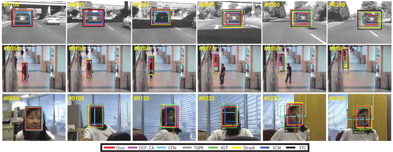
FIGURE 8. Qualitative results of the 8 trackers on the videos Car4 , Walking2 and Girl , in which the targets undergo large-scale variations.
