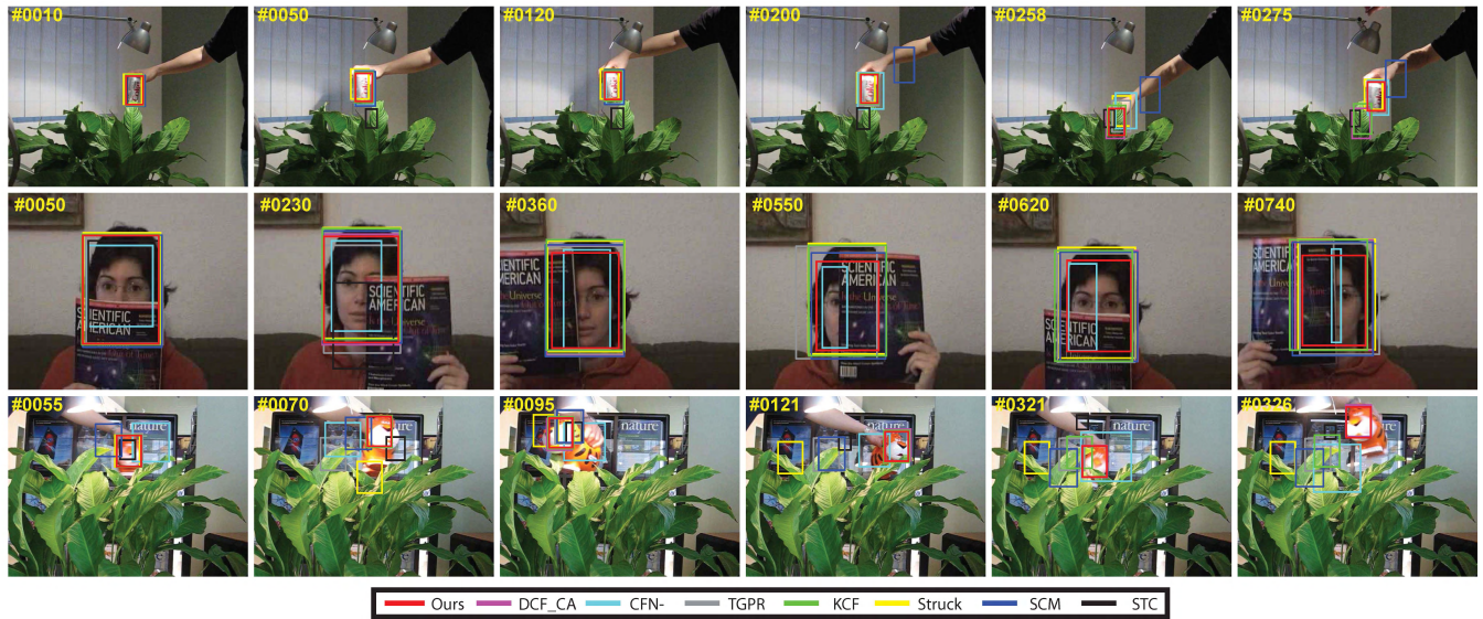
FIGURE 9. Qualitative results of the 8 trackers on the videos Coke , FaceOcc1 and Tiger1 , in which the targets undergo large-scale occlusions.
