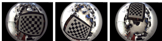
FIGURE 4. Example of calibration images with chessboard pattern in different positions and orientations.
