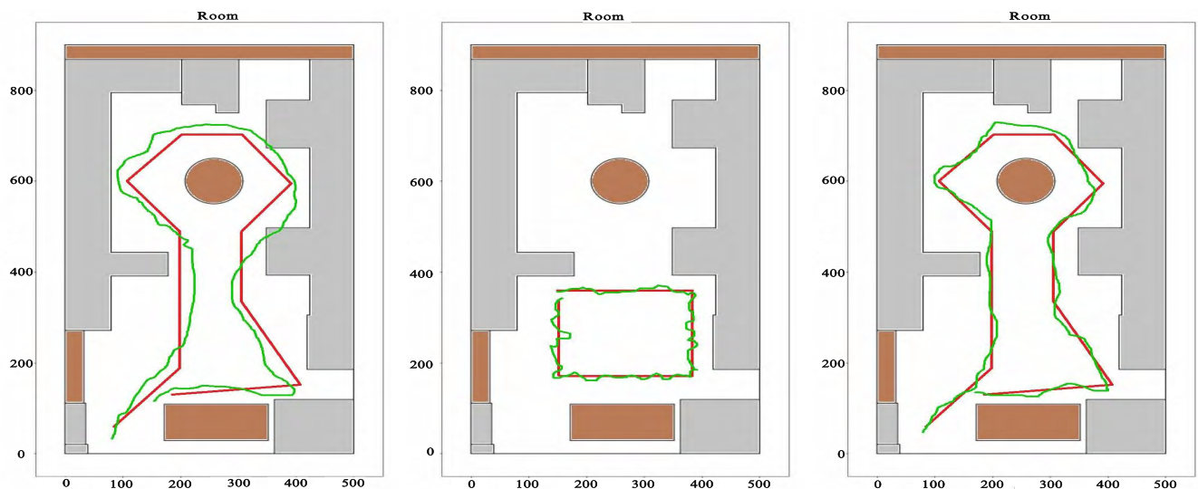
FIGURE 6. Example of trajectories extraction from WSN (left), Kinect (center) and Zenith camera (right). The red line shows the real path whereas the green line represents the estimated path. The WSN estimation accuracy is lesser than the one obtained from cameras. However, WSN coverage area is the largest of the sensors chosen. Finally, the Kinect range of detection constraints the potential applications. In the experiment, WSN is composed of 4 nodes located at the top corners of the room. Kinect sensor is located at 500, 300 in horizontal and vertical axis respectively and Zenith Camera is located in the room center at ceiling.
