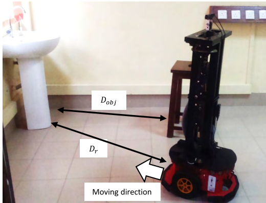
FIGURE 5. D_r and D_{obj} are explained in this figure. The robot is to move in the direction indicated by the white arrow. The distance from the robot to the nearest obstacle or the object of interest is denoted by D_r . The distance between the object of interest and the closest nearby object in the approach direction is denoted by D_{obj} .
