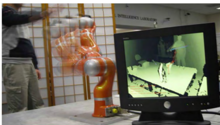
FIGURE 18. Avoidance of human-robot collision using RGB-D information [104].
