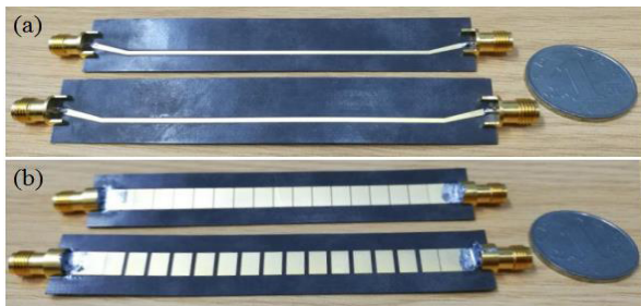
FIGURE 5. Two samples of the new structures with different interval i of 0.2mm and 1mm. (a)The top view of this two samples. (b)The bottom view of this two samples.
