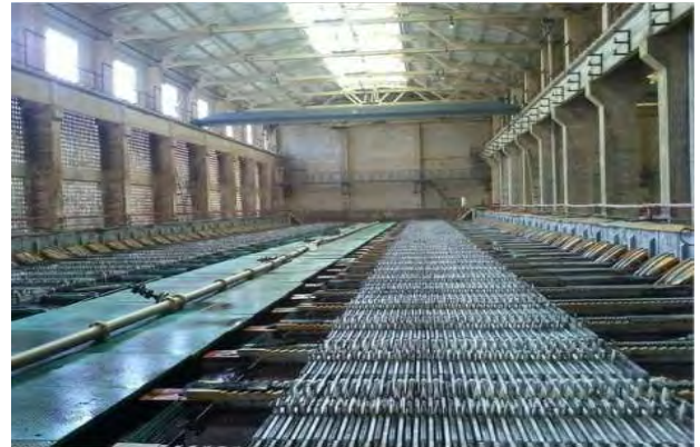
FIGURE 3. Electrowinning process in a zinc hydrometallurgy plant.
