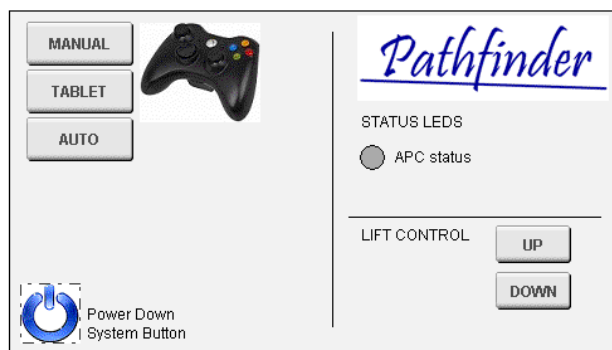
FIGURE 7. Main Pathfinder Service menu. 4,3 inch service touch panel mounted on the base platform allows users to switch between different control modes. For standard transport task definitions, Android application or Raspberry Pi display mounted on the cargo shelf can also be used.
