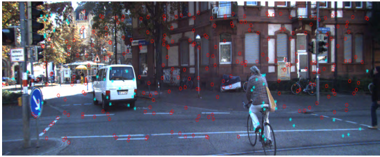
FIGURE 4. Illustration on dynamic and static key points for RANSAC based odometry method. The red circles represent the inliers which are classified as static points while the cyan stars represent the dynamic points which are removed to update the ego-motion.
