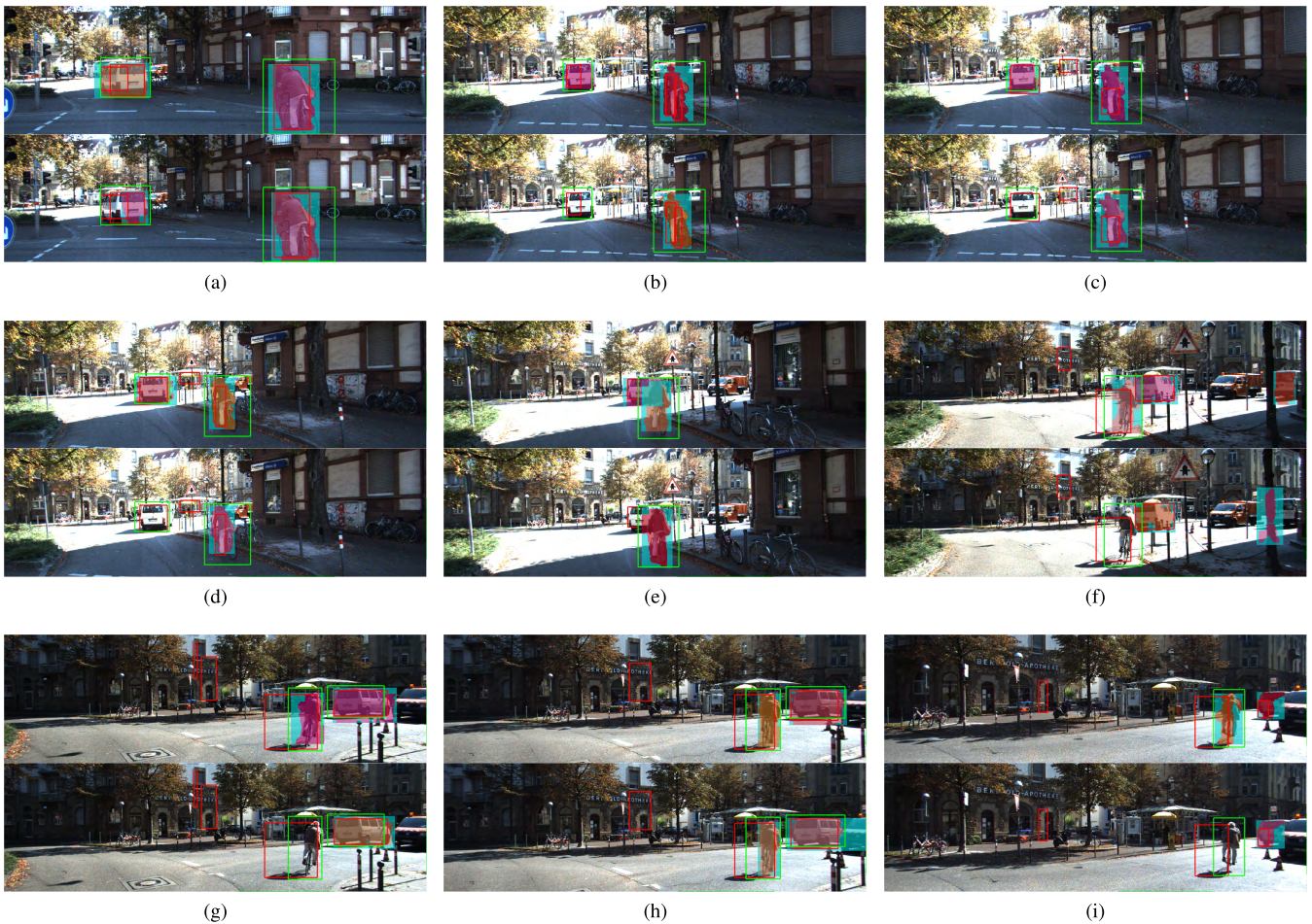
FIGURE 6. Typical qualitative results. The green bounding boxes are the 2D projections from ground truth 3D tracklets, the red ones are the detection results from baseline triTrack. Our method returns not only the bounding region in light cyan but also the object segmentation within it in relative darker colors. The first row of each subfigure shows the result of our method with Mahalanobis normalization while the second row without it.
