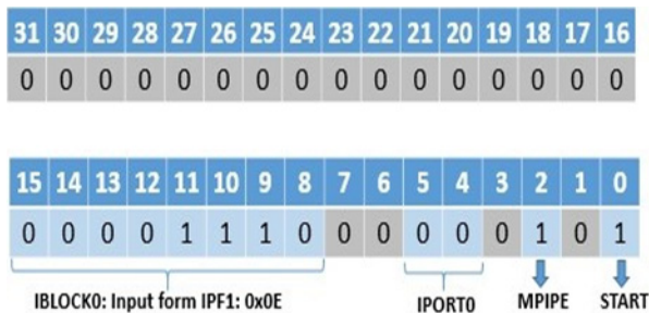
FIGURE 5. IIM configuration register PVP_IIM1_CFG.
