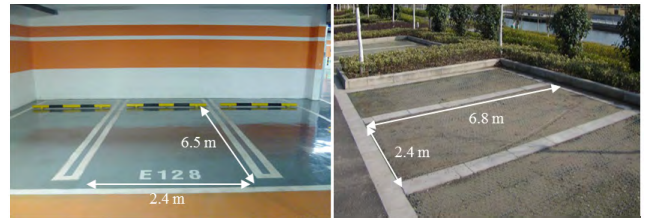
FIGURE 9. Common vertical parking spaces.
