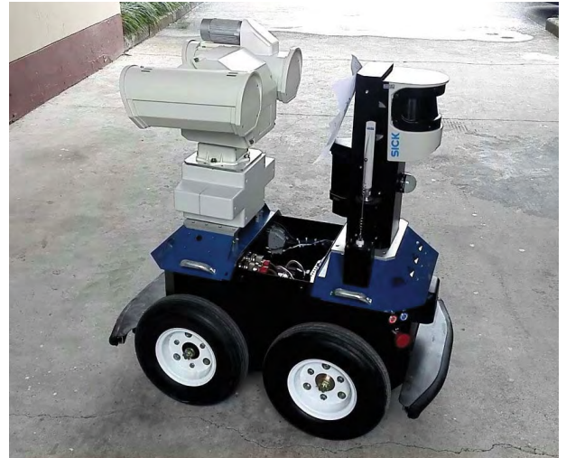
FIGURE 4. Skid steer mobile robot.
