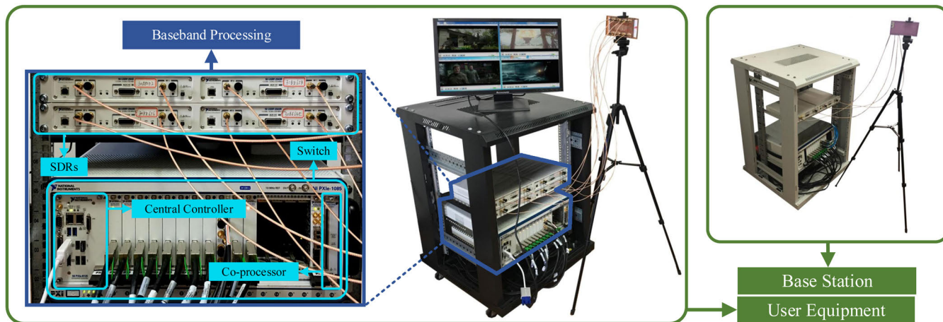
FIGURE 13. Photograph of the assembled testbed. Left: the photo of UE, including an 8-antenna module, a display screen, and baseband processing aspects. Right: the photo of BS, including a 4-antenna module and baseband processing aspects. The 8-element antenna module is located near the chassis, 1.5 meters away from the BS antennas.
