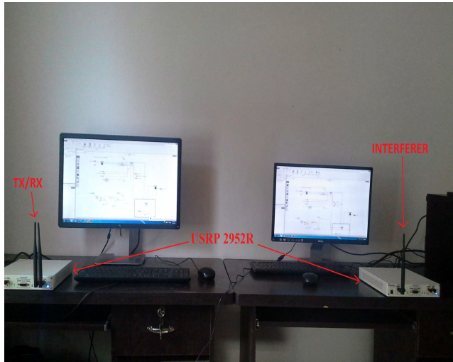
FIGURE 6. Experimental setup for IEEE 802.22 acts as an interferer.
