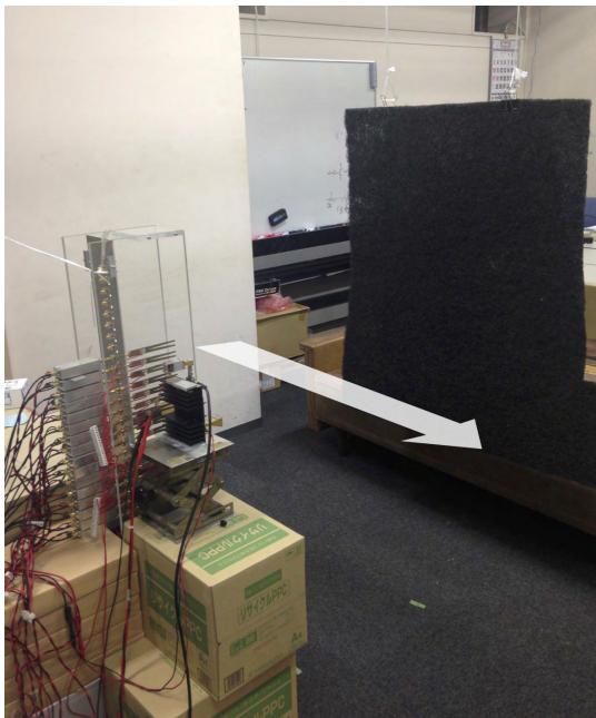
FIGURE 14. Experimental setup targeting a walking person. The target walks along the white arrow.
