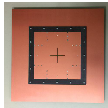
FIGURE 12. Photograph of the fabricated dual-polarized MPA.
