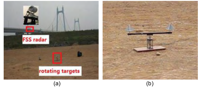
FIGURE 16. Outfield experiments of rotating targets. (a) FSS radar and the scenario of the outfield experiments. (b) Rotating targets.
