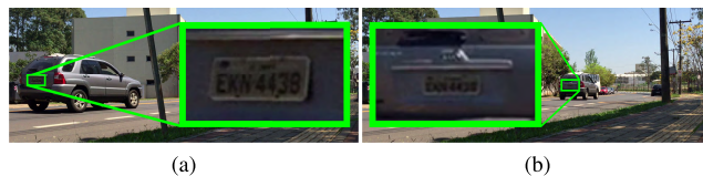
FIGURE 15. The license-plate alphanumerics are easily readable in the first video frames (a) but not in the last ones (b). We create ground-truth files with the initial frames, and the last frames are used to be reconstructed and recognized. The same zoom-in factor was applied to the license plates in (a) and (b).
