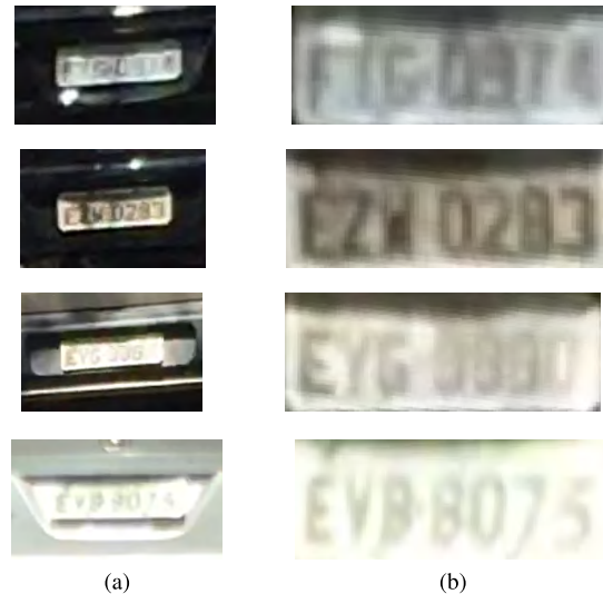
FIGURE 2. Output examples of the proposed framework. In (a), single frames with low-quality resolution. In (b), five consecutive frames are combined into a super-resolved image, richer in details.
