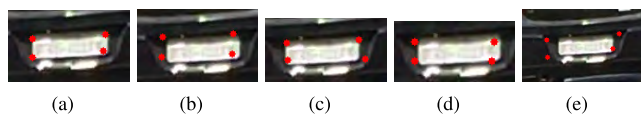
FIGURE 19. Examples of an input video tracked by PyrLK (a), PyrDense (b), SIFT (c), SURF (d) and ORB (e).
