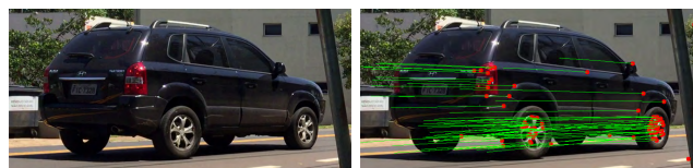
FIGURE 8. PyrLK feature tracker to estimate the optical flow.
