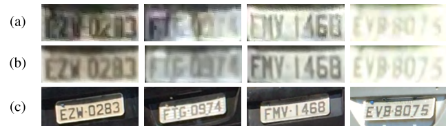
FIGURE 23. Quality of the reconstruction applied to frames with illumination and shadow issues. In (a), the initial frame without super-resolution. Then, the results for GSR_4 (b). In (c), a frame with a good resolution of the license plate.
