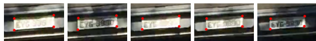
FIGURE 18. Cast shadows may impact the tracking step. The red dots show that PyrLK and PyrDense could track the frames even with a different lighting condition in each consecutive frame.
