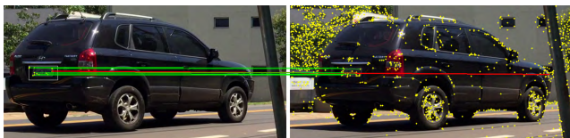
FIGURE 10. Tracking using SIFT. The white polygon is the region around the license plate in F_k . Yellow dots are the SIFT keypoints inside the small region in F_k and in the entire image F_{k+1} . Green lines are matches between the frames. The red line is an incorrect match that will not be used.
