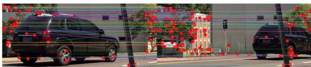
FIGURE 4. Matches between pairs of keypoints found by SIFT.
