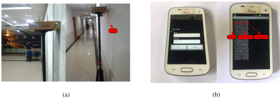
FIGURE 2. Hardware on WLAN platform. (a) Deployed APs. (b) Developed software.
