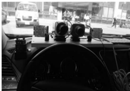
FIGURE 8. Driver monitoring cameras mounted on car dashboard [124].
