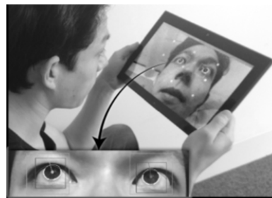
FIGURE 9. Eye tracking implemented in near real-time on a tablet. The tracking algorithm uses cascade classifiers and shape-based approaches to determine the eye region and centers. Elliptical model-fitting and 3D back-projections are then used to determine the eye optical axes and point-of-gaze [18].
