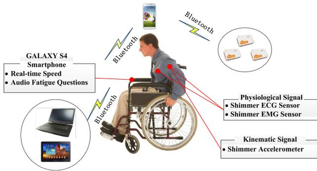
FIGURE 2. Diagram of hardware deployment and communication between layers.
