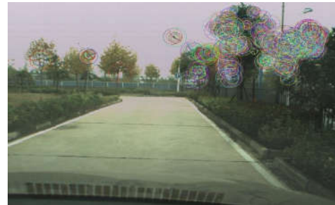
FIGURE 5. Extraction of ORB local features.
