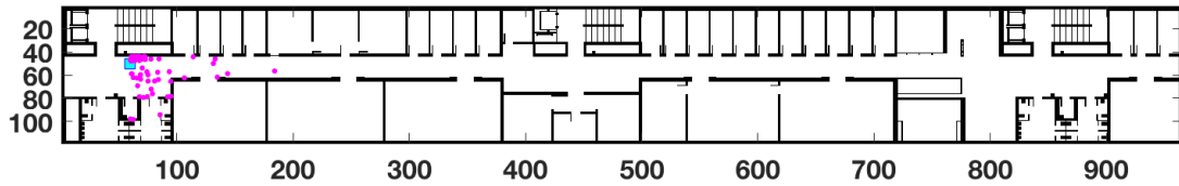
FIGURE 7. Laser scan with 50% of contamination. All units in cells. Robot's location in blue square.
