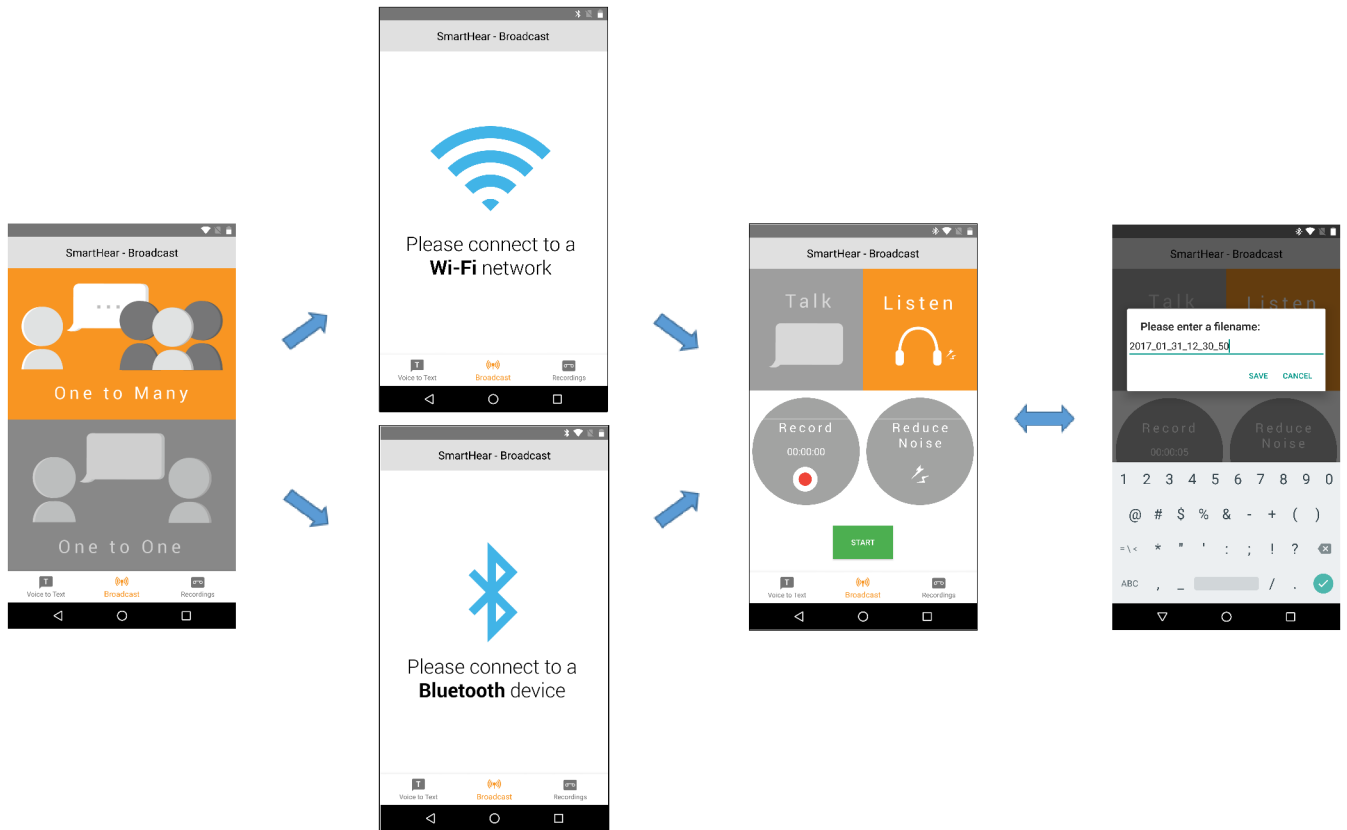
FIGURE 6. SmartHear’s user interfaces related to the “Broadcast” function. The initial screen prompts the user to choose between “One to Many” and “One to One.” After choosing “One to Many” (respectively, “One to One”), the second screen prompts the user to connect to WiFi (respectively, Bluetooth). Once connected, the third screen is displayed, which consists of various control configurations for the voice transmission session. The fourth screen shows the text box dialog which is prompted at the end of a recording session.
