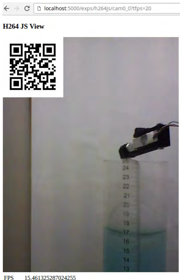
FIGURE 6. Interactive live-stream with an embedded QR timestamp to measure the true capture-render delay.
