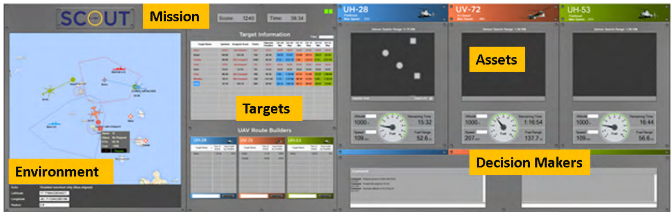
FIGURE 9. Supervisory Control Operations User Testbed (SCOUT): Left screen - shows the position of the UASs, targets in Google Maps, and information about the UASs and targets; Right screen - shows the sensor feed, UAS information (speed, altitude), and two chat windows for INTEL updates and commands [85].
