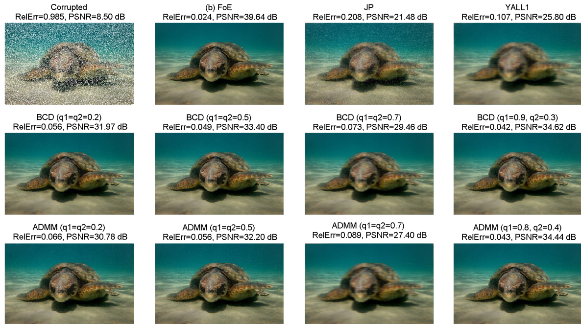
FIGURE 4. Restoration of a 318 \times 500 image corrupted by salt-and-pepper impulsive noise using the compared methods. (a) Corrupted image with salt-and-pepper impulsive noise (30% of the pixels are corrupted). (b) FoE (PSNR = 39.64 dB). (c) JP (PSNR = 21.48 dB). (d) YALL1 (PSNR = 25.80 dB). (e)–(h) Proposed BCD method for different q_1 and q_2 (best PSNR = 34.62 dB). (i)–(l) Proposed ADMM method for different q_1 and q_2 (best PSNR = 34.44 dB). Note: Even though FoE is significantly effective, it requires the mask of the corruption.
