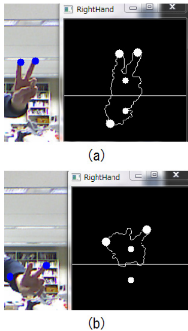
FIGURE 16. The effect of direction of the palm of the hand to fingertip detection (a) the palm of the hand facing frontally to the Kinect (b) the palm facing another direction.
