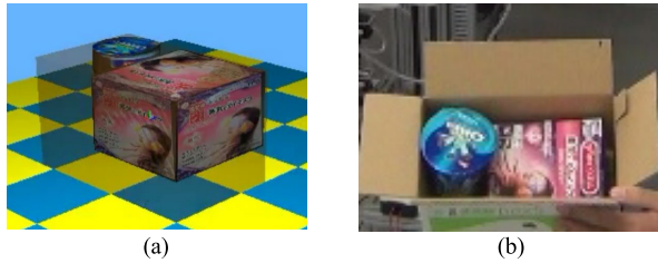
FIGURE 18. The comparison of the planned deployment and the executed one. (The filling rate is 37.54).
