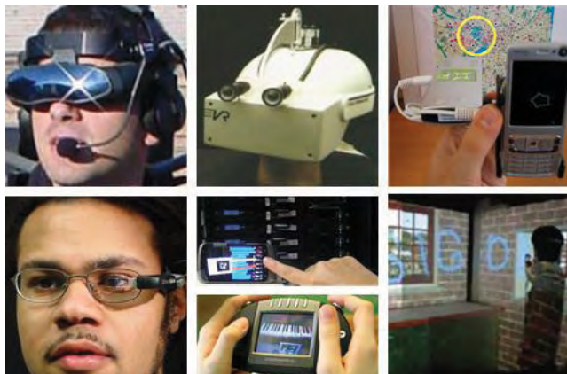
FIGURE 6. Several display ways in MAR. Optical see-through display (Left): Sony Glasstron LDI-D100B and MicroOptical Clip-on; Video see-through display (Middle): two camera mounted HMD of UNC, mobile phone [88] and PDA [53]; Surface project display (Right): mobile camera projector [174] and laser projector [175].
