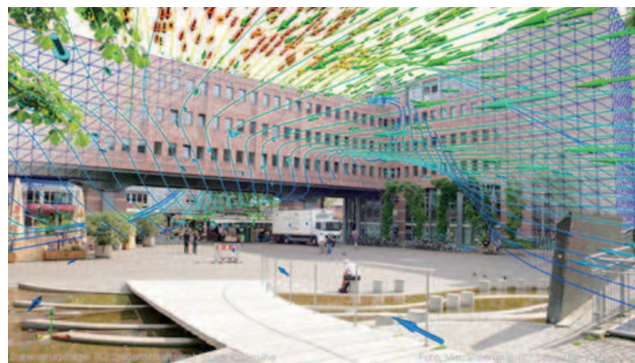
FIGURE 3. Visualization of a numerical flow field with real buildings makes the influence of the building on wind movement easily understood. (source: http://emcl.iwr.uni-heidelberg.de/researchsv.html )
