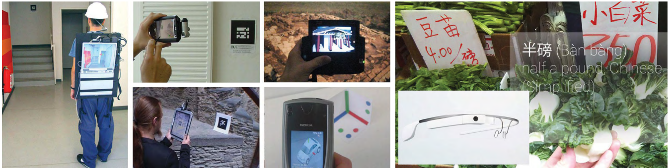
FIGURE 5. Several mobile devices used in MAR applications. Left: Notebook computer [114]; Middle: PDA [115], Tablet PC [116], UMPC [117], and mobile phone [118]; Right: Google Glass [91].
