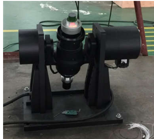
FIGURE 11. Single-axis rotary table layout of triaxially orthogonal coils.
