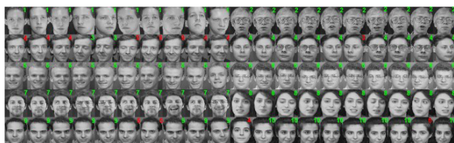
FIGURE 11. Clustering results of our method on Olivetti Face Database for the first 100 images. Digit on face represents cluster label, faces with the same digit belong to the same cluster, faces with green digit are correct clustering, and faces with red digit are wrong clustering.
