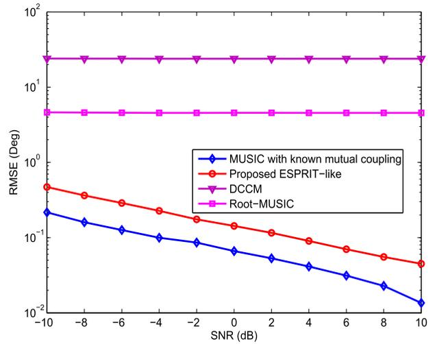
FIGURE 8. RMSE of DOA estimation of proposed ESPRIT-like algorithm versus SNR (Case-II).
