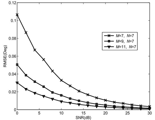
FIGURE 4. RMSE of DOA estimation of the proposed ESPRIT-like algorithm versus SNR for different  $M$  (Case-I).
