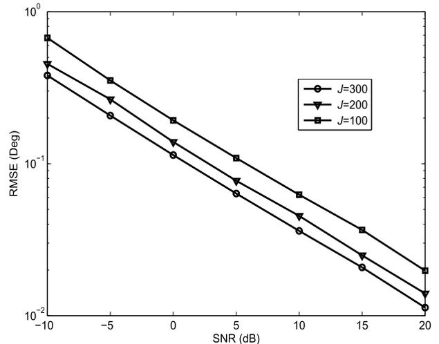
FIGURE 9. RMSE of DOA estimation of the proposed ESPRIT-like algorithm versus SNR for different numbers of snapshots  $J$  (Case-II).
