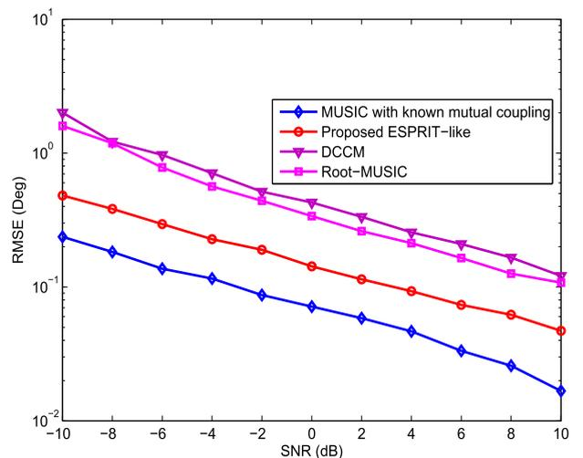
FIGURE 5. Comparison of the RMSEs of DOA estimation of different methods versus SNR (Case-I).
