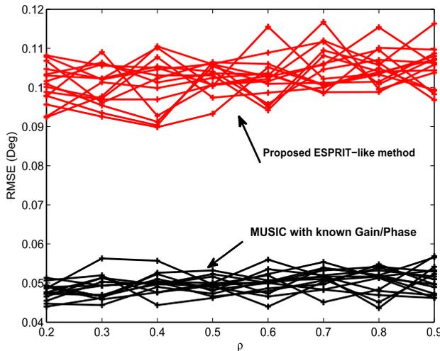
FIGURE 10. Comparison of the RMSEs of DOA estimation versus  $\rho$  with  $\phi \in [\pi/10, \pi]$  (Case-II).
