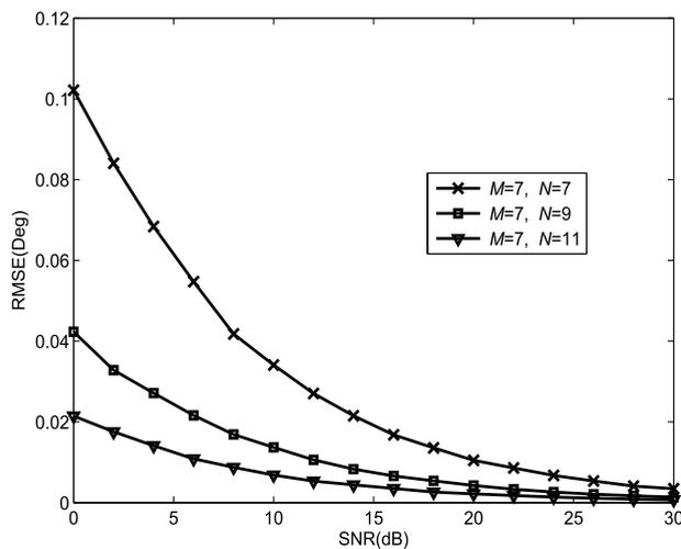
FIGURE 3. RMSE of DOA estimation of the proposed ESPRIT-like algorithm versus SNR for different  $N$  (Case-I).
