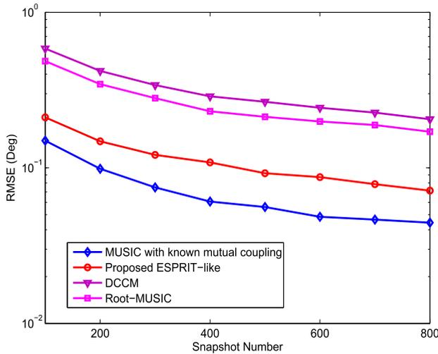
FIGURE 6. RMSE of DOA estimation of different methods versus the number of snapshots (Case-I).
