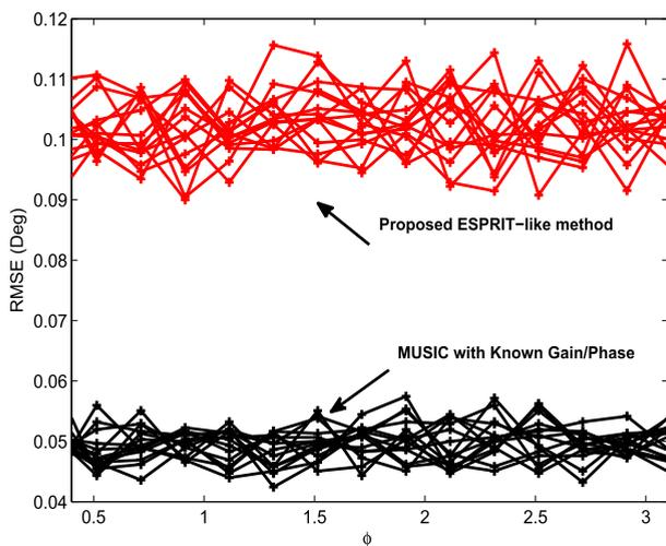
FIGURE 11. Comparison of the RMSEs of DOA estimation versus  $\phi$  with  $\rho \in [0.2, 0.9]$  (Case-II).
