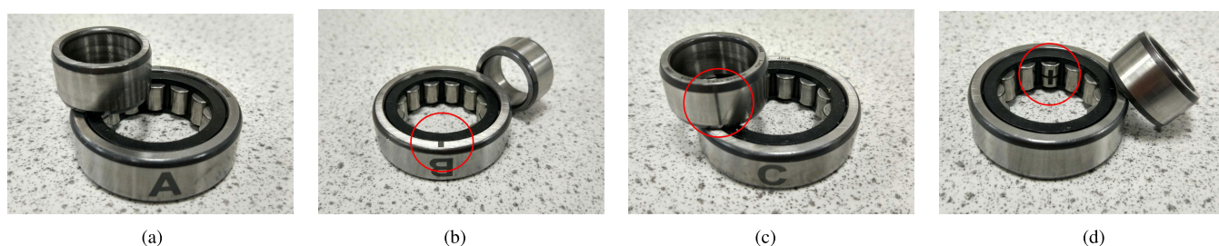
FIGURE 4. Four conditions of the experimental bearings. (a) Normal bearing A as reference. (b) Bearing B with outer race defect. (c) Bearing C with inner race defect. (d) Bearing D with roller defect.
