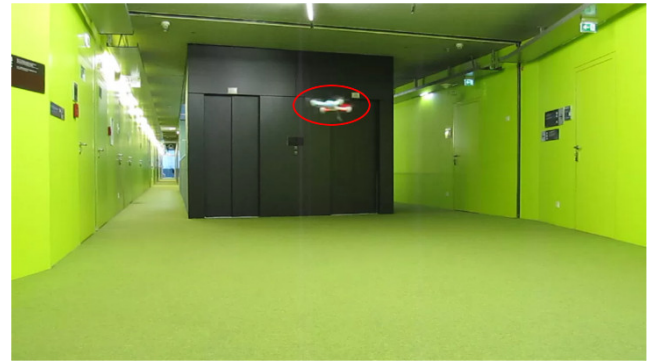
FIGURE 18. Measurement scenario UAV flying indoors. The UAV is a fast target and the scenario produces lots of multi-path detections.
