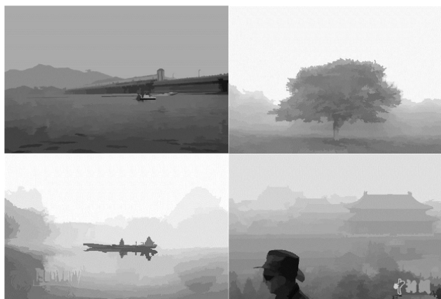
FIGURE 2. Segmentation results by mean shift algorithm, different regions are distinguished by different grey values, from left to right: wharf, tree, boat, and man_in_haze.
