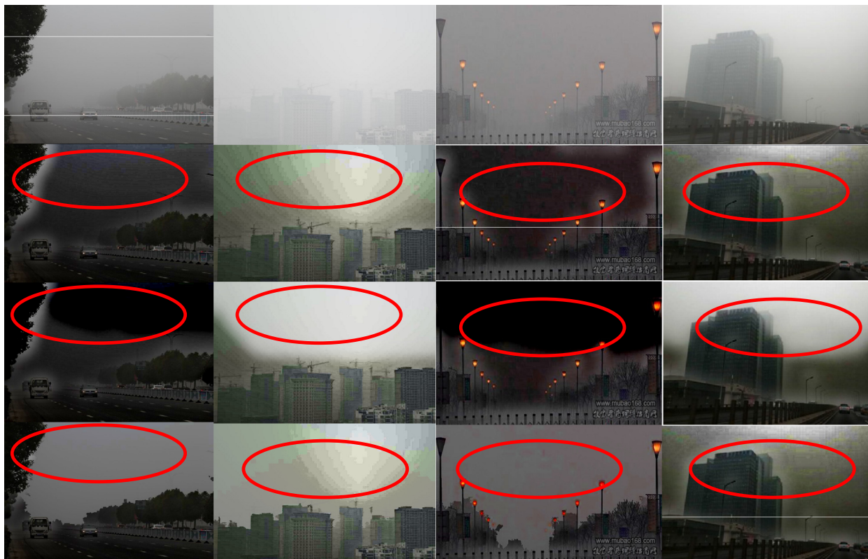
FIGURE 10. Comparison of dehazed images, the first row shows the input hazy image, the second row shows the dehazed images of the method in [6], the third row shows the dehazed images of the method in [7], the fourth row shows the dehazed images of the proposed method, from left to right: road, city, streetlight, and building.
