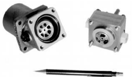
FIGURE 11. Port plate and cylinder port matching construction of NHT [23].
