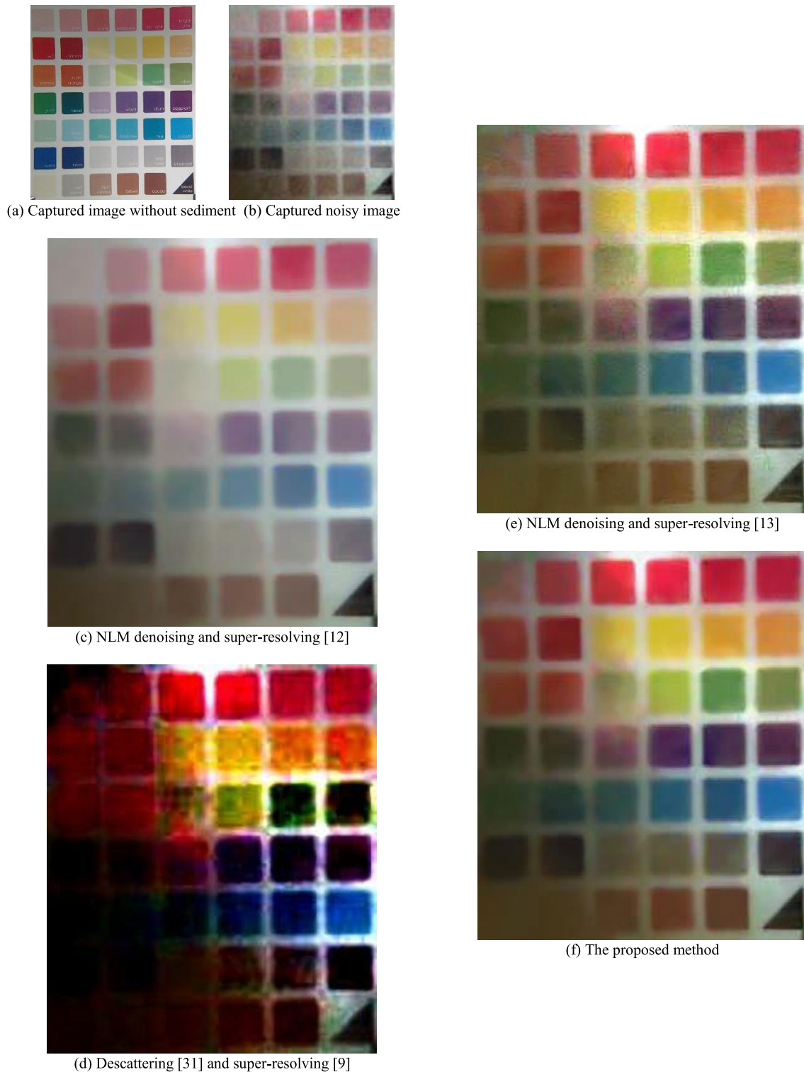
FIGURE 2. Simulation results of water tank. (a) Captured image without sediments and noise. (b) Captured image with 200 mg/L turbidity and additional noise. (c) Super-resolved result using the method in [12]. (d) Super-resolved result using the method in [9]. (e) Super-resolved result using the method in [13]. (f) Super-resolved result using the proposed method. (a) Captured image without sediment (b) Captured noisy image. (c) NLM denoising and super-resolving [12]. (d) Descattering [31] and super-resolving [9]. (e) NLM denoising and super-resolving [13]. (f) The proposed method.
