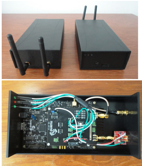
FIGURE 14. An SDR platform from Nuand was used to build the fully autonomous cooperative routing scheme. The platform houses a 40-KLE Altera Cyclone IV FPGA, a Cypress micro-controller unit (MCU), and a reconfigurable RF chipset from Lime Microsystems. An RF amplifier from Texas Instruments was also annexed to the platform. The OFDM PHY was built on the FPGA, while the rest of the protocol stack runs on the MCU.
