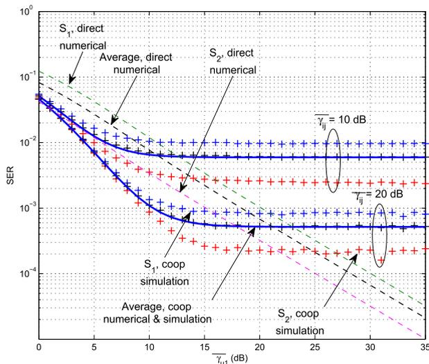
**FIGURE 8.** SER of the cooperative system in non-identically distributed Rician channels with BPSK,  $n_R = 1$ ,  $K_1 = K_2 = 2$ ,  $\bar{\gamma}_{ij} = 10$  and  $20$  dB,  $\bar{\gamma}_{u2} = \bar{\gamma}_{u1} + 5$  dB. Plus markers indicate simulation results.
