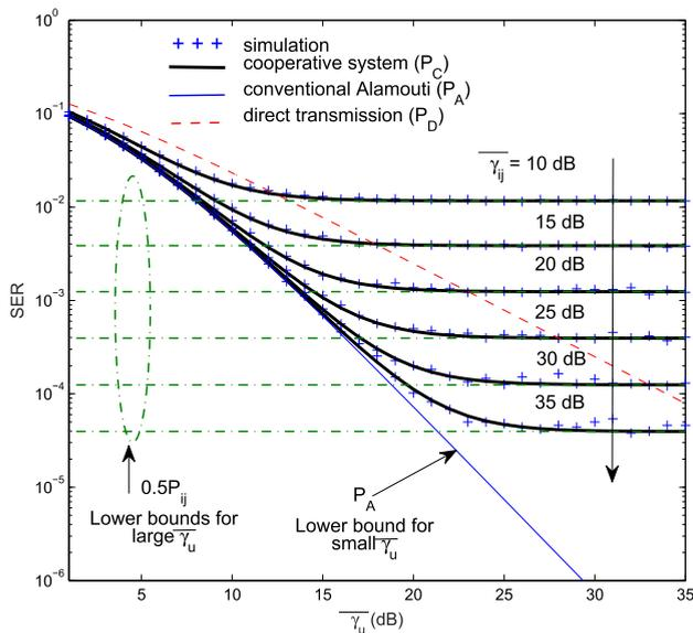
FIGURE 6. Error performances of the direct transmission system, cooperative system, and conventional Alamouti system with BPSK,  $n_R = 1$ , and identically distributed Rayleigh fading channels. Solid and dashed curves show the numerical analysis, while plus sign markers show the simulations.
