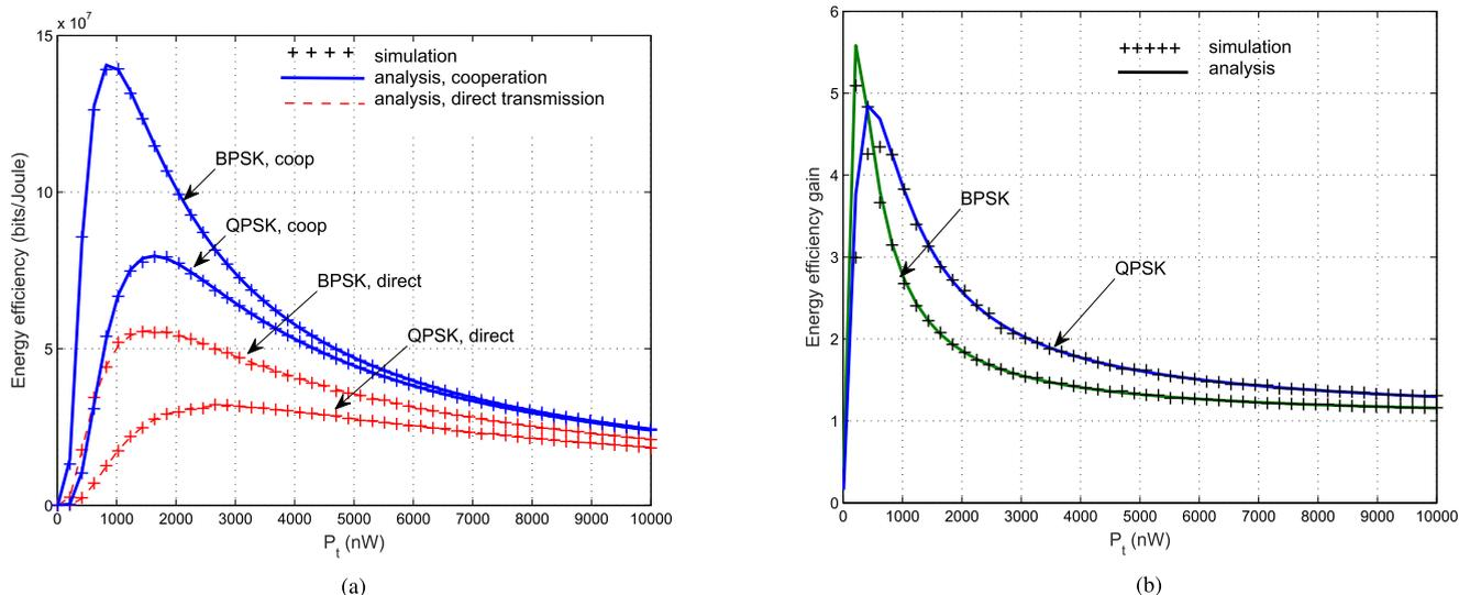
FIGURE 12. Numerical and simulated  $EE$  and  $G_{EE}$  as functions of the transmitted power  $\mathcal{P}_t$  in the cooperative communication and in the direct transmission. (a)  $EE$ . Dashed curves - direct transmission, solid - cooperation. Circle markers - BPSK,  $n_R = 1$ ; square - BPSK,  $n_R = 2$ . Plus markers - simulated cooperation, asterisks - simulated direct transmission. (b)  $G_{EE}$ .
