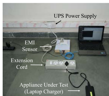
FIGURE 10. Block view of EMI sensor.
